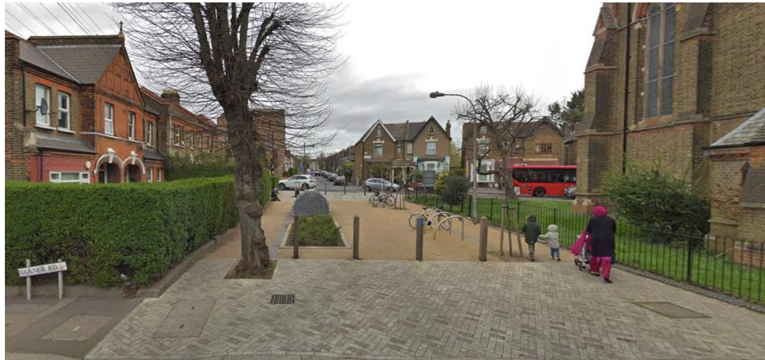
Modal filter removes through traffic, allowing walking and cycling and improving public realm
