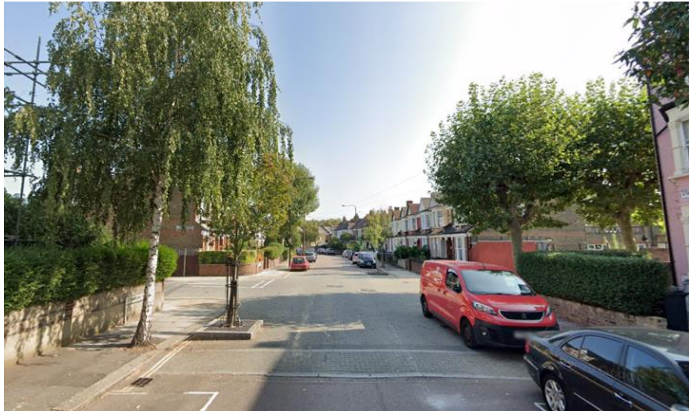
Raised plateau at junction slowing traffic and providing level crossing for pedestrians
