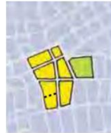
This street pattern then forms the basis for perimeter blocks which ensure that buildings contribute positively to the public realm.
